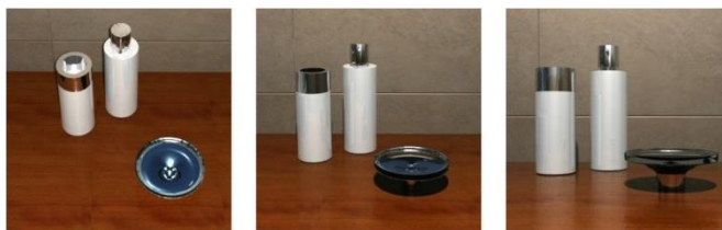
Reflection made by polished lacquered wood depending on view angle. Es. 0 deg refl = 10 e 90 deg refl = 100
